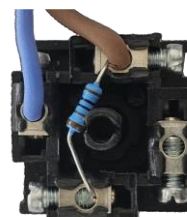
Resistor AER101 plugged in the pressure switch connection point 1 and 2
