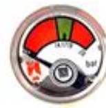
Pressure level is critical
