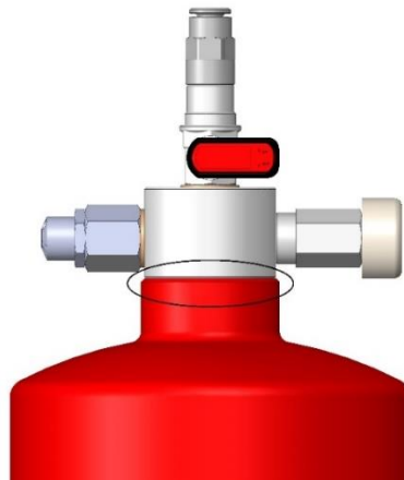
Connection between the cylinder neck ring and the valve
