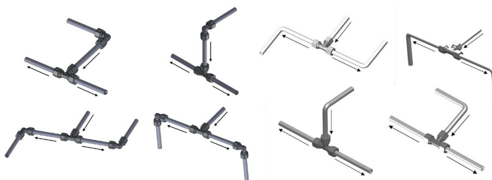
Acceptable ways of connections into a Tee
