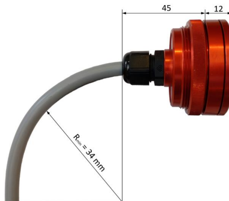
Minimal cable bending radius
