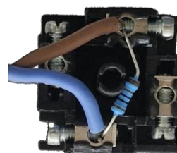
Resistor AER101 plugged in the pressure switch APS003 connection point 1 and 2
