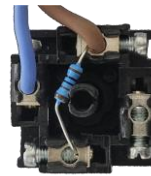
Resistor AER101 plugged in the pressure switch APS001 connection point 1 and 2
