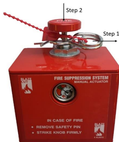
Procedure of manual activation
