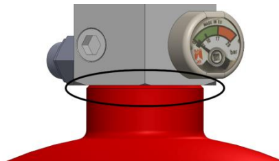
Connection between the cylinder neck ring and the valve
