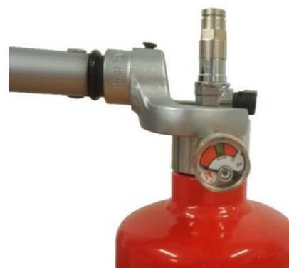
Assembly of the valve using a torque wrench
